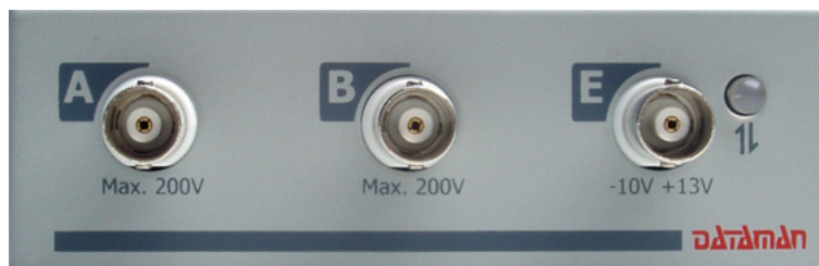
Fig. 2.1.1.3. – Front panel of the DATAMAN 770 series oscilloscope
