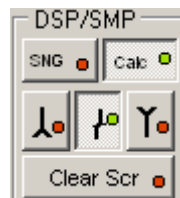
Fig. 4.6.1. – Waveform display mode controls
