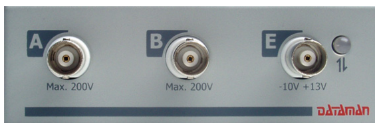
Fig. 2.1.1.3. – Front panel of the DATAMAN 770 series oscilloscope
