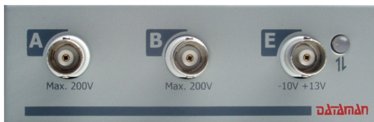
Fig. 2.1.1.1. – Front panel of the DATAMAN 570 series oscilloscope
