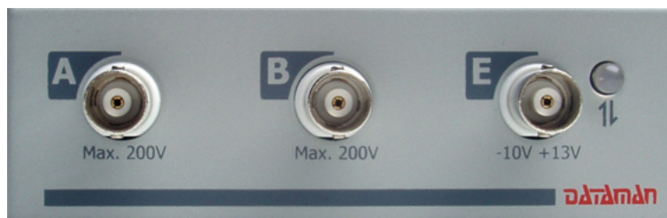
Fig. 2.1.1.2. – Front panel of the DATAMAN 520 series oscilloscope
