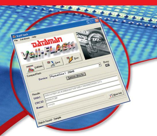
Dataman Vali-Flash is a PC based validator designed for calculating the CRC-32 and SHA-1 signatures for CompactFlash® memory devices. Vali-Flash offers many exciting and advanced features as shown below.
