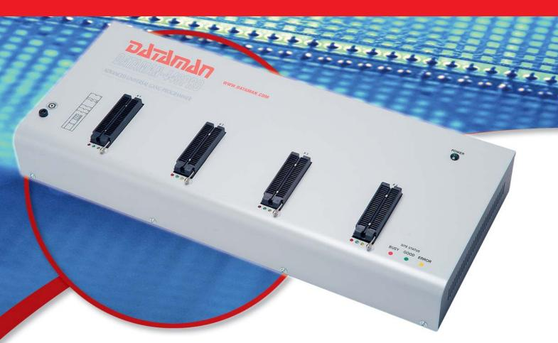
The Dataman 448Pro is a PC based gang programmer featuring four independent universal programming modules and USB 2.0 connectivity. Supporting over 20,000 devices with new support added monthly, the Dataman 448Pro can program without the need for a family-specific modules, giving you the freedom to choose the optimal device for your design.
