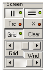
Fig. 4.1.3.1. – The cursors and grid controls
