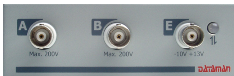
Fig. 3.1.1.3. – Front panel of the DATAMAN 770 series oscilloscope
