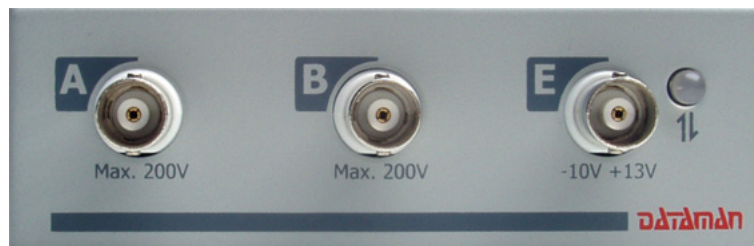
Fig. 3.1.1.1. – Front panel of the DATAMAN 570 series oscilloscope
