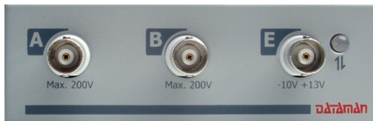
Fig. 3.1.1.2. – Front panel of the DATAMAN 520 series oscilloscope
