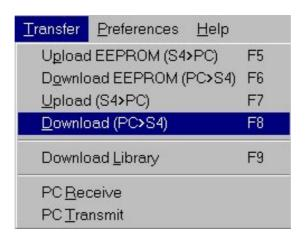
Intel Hex and Motorola S format files will download automatically after the above procedure has been carried out. However, Binary and ASCII files require file ranges to be entered before the file can be downloaded. The File Examine feature will inform the user of the range of the data.
