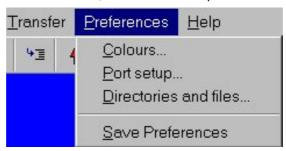
Please check that the <u>Parity</u> is set to **None**, <u>Data bits</u> to **8** and <u>Stop bits</u> to **one** and that the Baud rate is set to the same Baud rate that you have the *S4 Validator* set to in the setup function. Remember that the Baud rate settings here **MUST** match those of the *S4 Validator* in order to communicate with the PC. When the Com port is correctly configured, left click on OK and return to the main screen.
