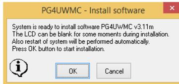
During update process, control program of Stand-Alone programmer is closed, LCD panel can be blank for some moments and after installation is complete, automatic restart of standalone programmer will be performed. Whole process should not exceed time of 1-2 minutes.
