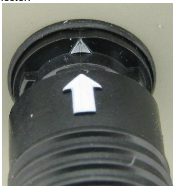
Arrows on power supply connectors
