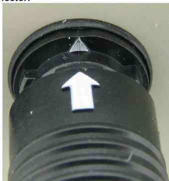
Arrows on power supply connectors
