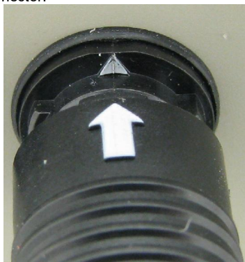
Arrows on power supply connectors
