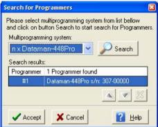
In combo box "Multiprogramming system" select Dataman-448Pro and click on "Search" button. After end of successful search click on "Accept" button to finish Search of programmer.
