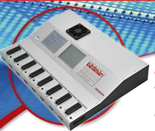
The Dataman 848Pro2 is a super fast stand-alone gang programmer with eight independent 48-pin ZIF sockets, ISP capabilities and internal control PC driven by Windows Embedded 8.1 Industry Pro. The 848Pro2 is built to meet the demands of super fast high volume production programming with minimal operator effort.
