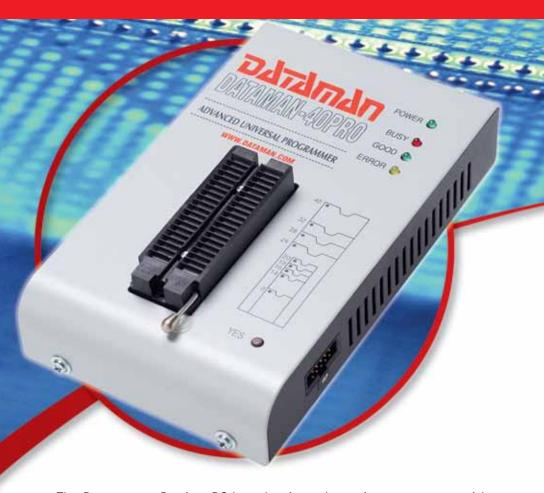
The Dataman 40Pro is a PC based universal 40-pin programmer with ISP capabilities and USB 2.0 connectivity. The 40Pro is built to meet the demands of development labs and field engineers for universal and portable programming.
