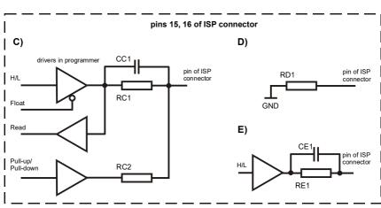
RA1 180R, RA2 1k3, RA3 22k, RB1 10k, RB2 10k, CC1 1n, RC1 1k3, RC2 22k, RD1 22k, CE1 1n, RE1 1k3,
