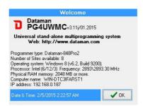
Welcome screen is displayed on standalone's build-in LCD screen after successful starting of standalone control software. The screen can be also displayed by using menu command 'Help / About'. Welcome screen contains following basic information:
