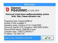
Welcome screen is displayed on Stand-Alone build-in LCD screen after successful starting of standalone control software. The screen can also be displayed by using menu command **Help / About** more information see **Help / About**.
